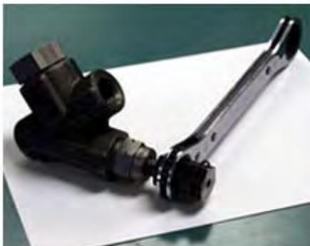
To ensure they could maintain the equipment and prevent worker injury, the team also created a new tool. The design of their new wrench allows steam to vent through it when the drain on a steam trap is opened. This new wrench makes trap repairs much safer by eliminating the potential for steam burns. The design of the wrench also ensures a snug fit and is easy to use in confined spaces, making for a smooth, safe and trouble-free operation.
