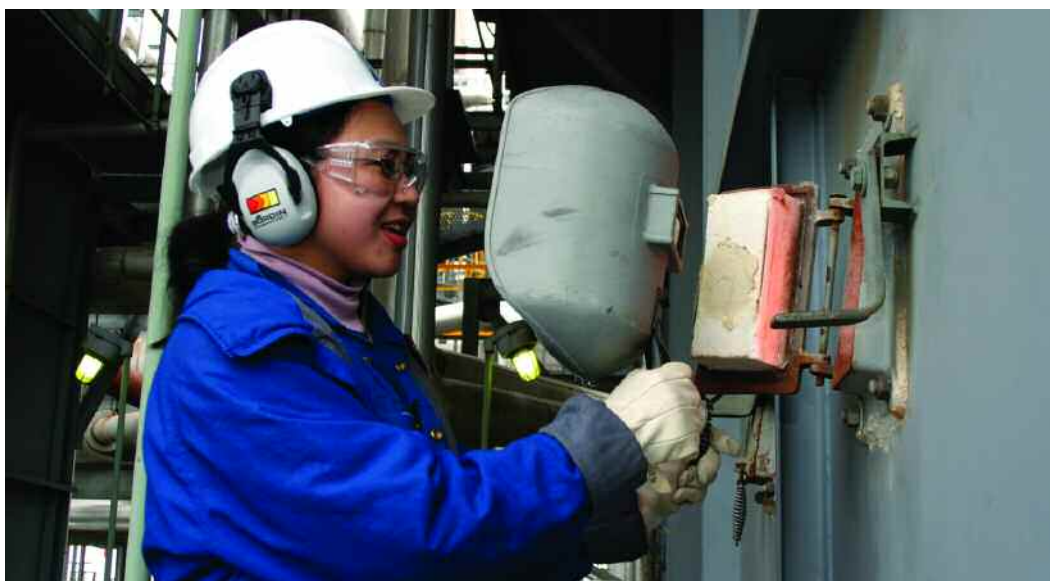
A NOVA Chemicals employee wears personal protective equipment including a hardhat, earmuffs, safety goggles, flame retardant jacket and leather gloves as she views the firebox of a cracking furnace through an inspection port. The welder's mask provides additional eye protection.
